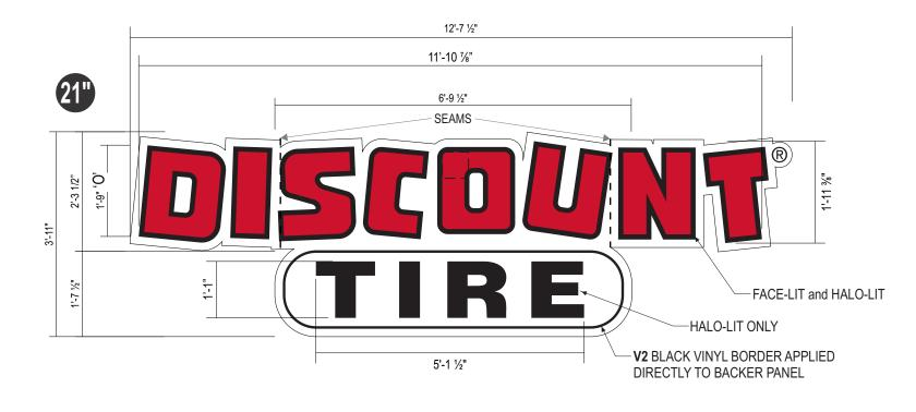
CUSTOM FABRICATED "DISCOUNT TIRE "FACE-LIT / HALO ILLUMINATED CHANNEL LETTERS W/BACKER PANEL - EXTERIOR
