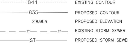
EXISTING CONTOUR -835------ PROPOSED CONTOUR PROPOSED ELEVATION ------ PROPOSED STORM SEWER
